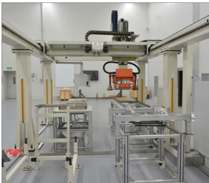
图4 自动折弯设备 Fig.4 Automated bending equipment
