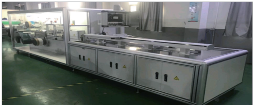
图7 芯材拉挤设备 Fig.7 Automated pultrusion molding equipment of radius fillers
